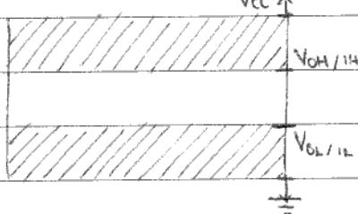
Each input is designed so that any voltage below  $V_{IL}$  is regarded as logic 0 and any voltage above  $V_{IH}$  is regarded as logic 1. Same goes for output.
